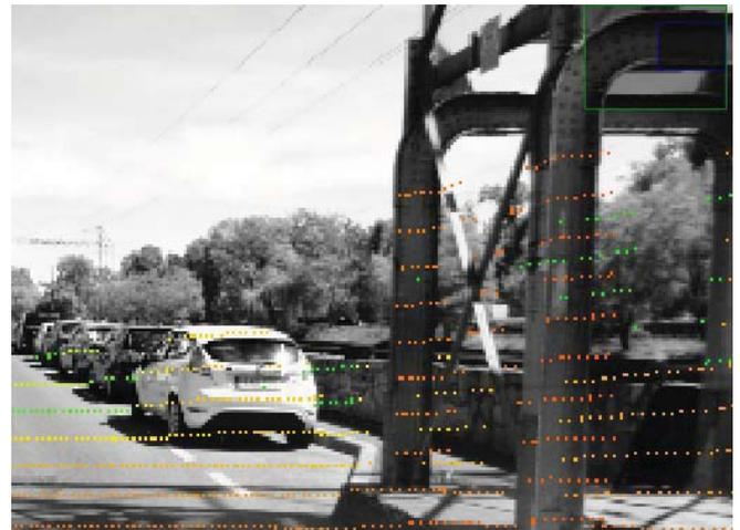
Figure 8. Corrected cross-calibration and projection of LIDAR data on image
